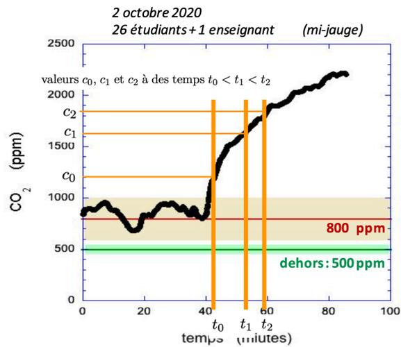
$$\hat{R} = R_{\text{ref}} \frac{\log\left(\frac{c_2 - c_0}{c_1 - c_0} - 1\right) - \log\left(\frac{t_2 - t_0}{t_1 - t_0} - 1\right)}{\log\left(\frac{1 - e^{-R_{\text{ref}}(t_2 - t_0)}}{1 - e^{-R_{\text{ref}}(t_1 - t_0)}} - 1\right) - \log\left(\frac{t_2 - t_0}{t_1 - t_0} - 1\right)}$$
